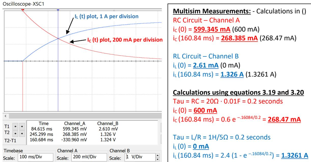
Figure 3.21: Multisim oscilloscope current measurements compared to calculations.
