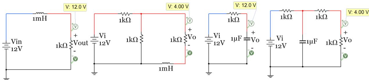
**Figure 3.33: Passive Low Pass Filter (LPF) Circuit Examples**
