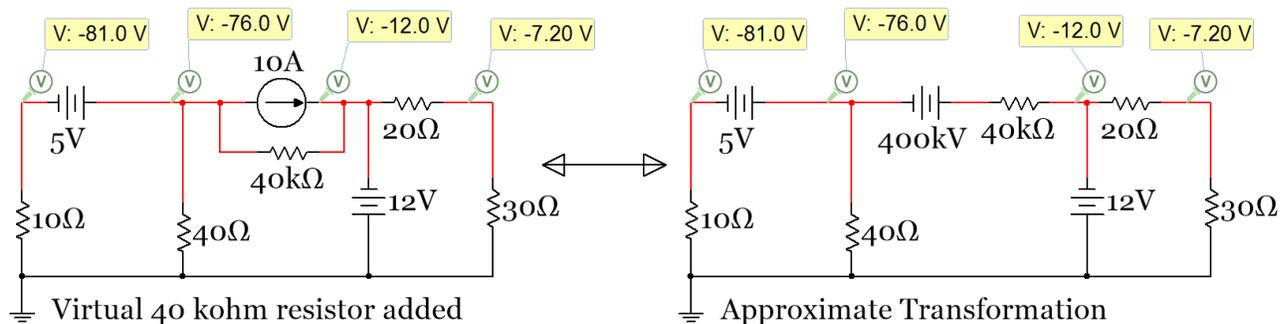
**Figure 2.8: Approximate Source Transformation of Circuit in Example 2.4**
