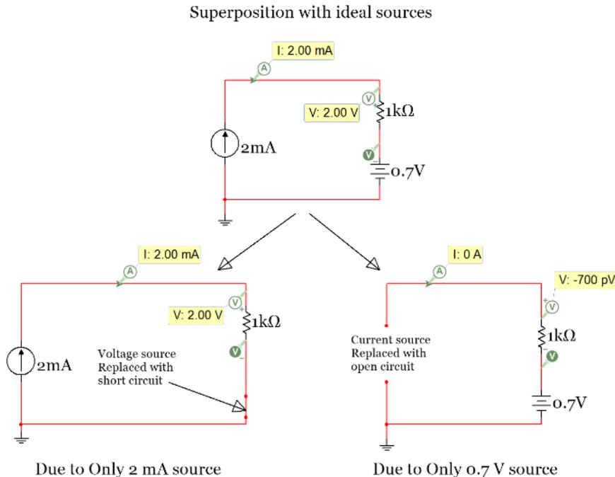
**Figure 2.34: Example of Superposition with Ideal Sources**
