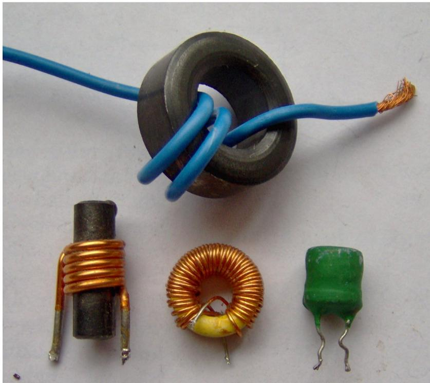
Figure 3.8: Inductor examples. Photo © FDominec and used under a CC BY-SA 3.0 license: [https://commons.wikimedia.org/wiki/File:Electronic\\_component\\_inductors.jpg](https://commons.wikimedia.org/wiki/File:Electronic_component_inductors.jpg)
