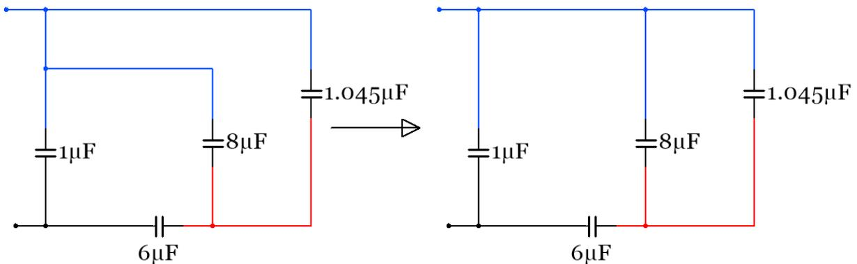
Figure 3.17: Simplification of Step 3 Circuit in [Figure 3.16](#)
