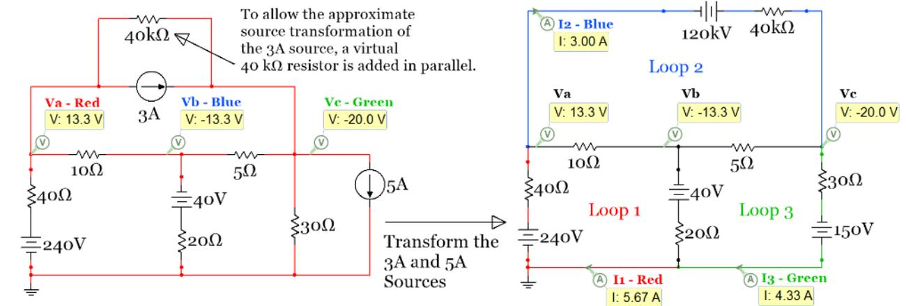
Figure 2.28: Circuit and Matrix for Example 2.14
