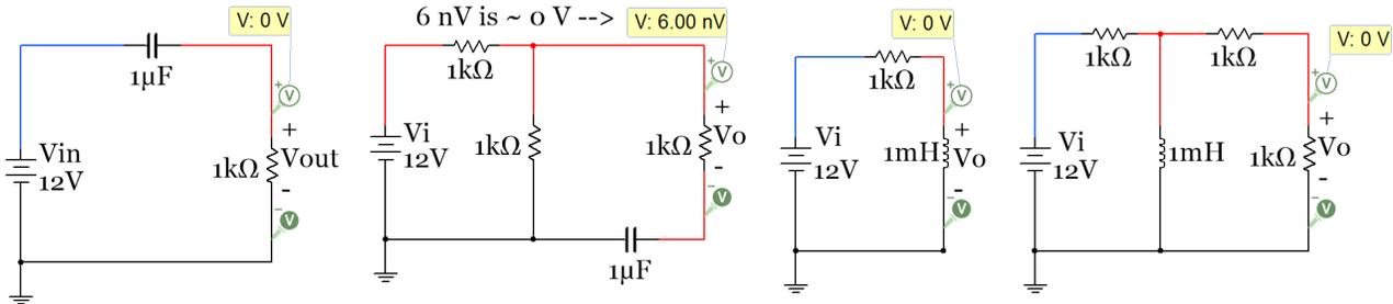
**Figure 3.32: Passive High Pass Filter (HPF) Circuit Examples**
