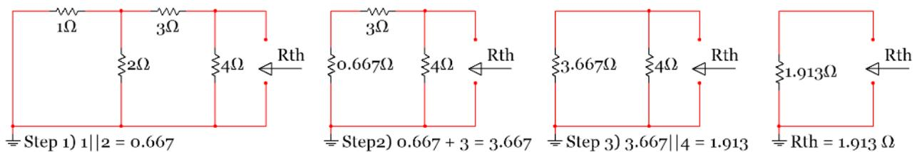
**Figure 2.60: Sub-Problem 1 - Rth Calculation using Method 1**
