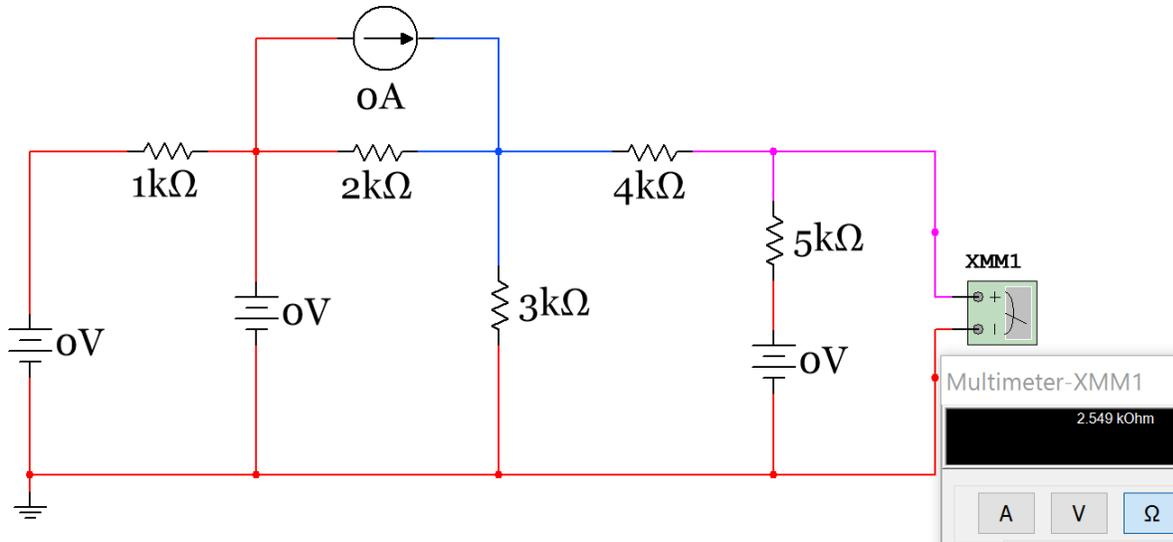
Figure 2.52: Multisim verification of  $R_{th}$  in Example 1.19 (done by plugging in zero for all sources instead of replacing with shorts and opens). This method is often easier to do quickly in Multisim.
