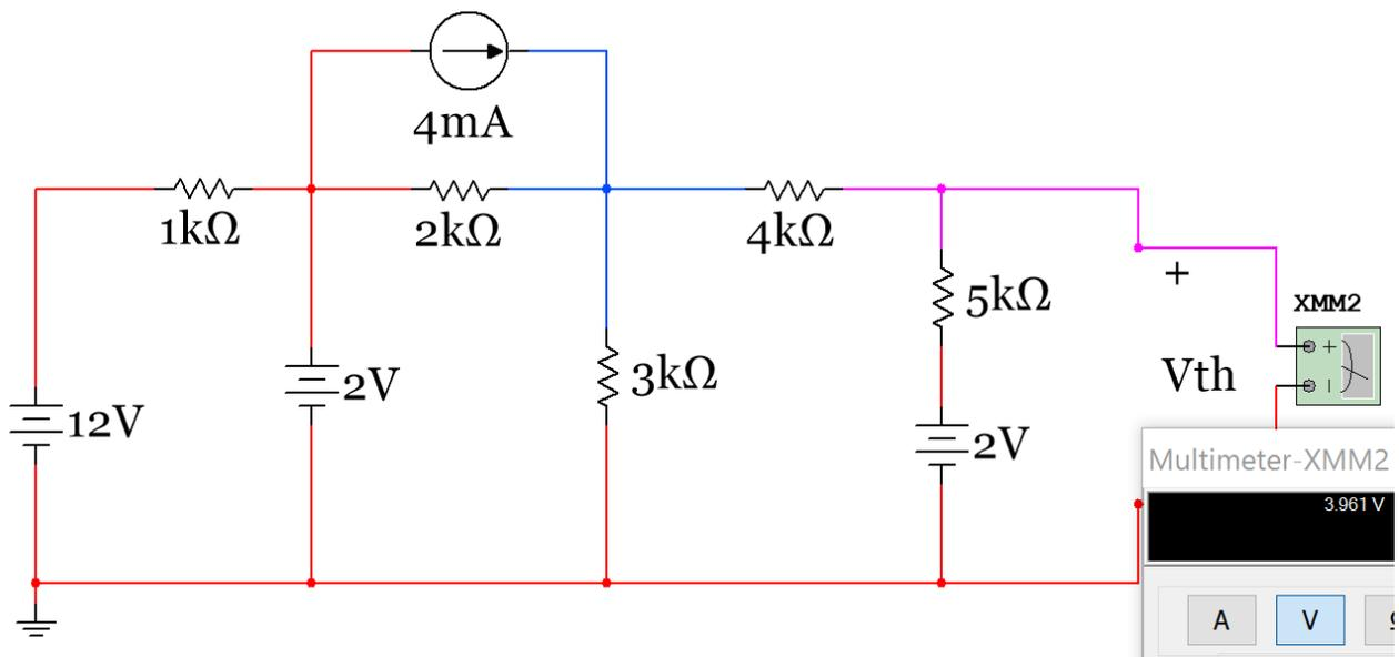
Figure 2.53: Multisim verification of  $V_{th}$  in Example 1.19.
